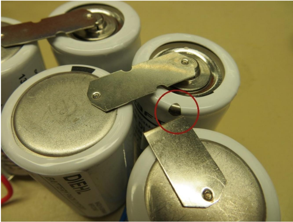
DEFECTIVE CELL INSULATION: EXAMPLE 1 FIGURE 5002
