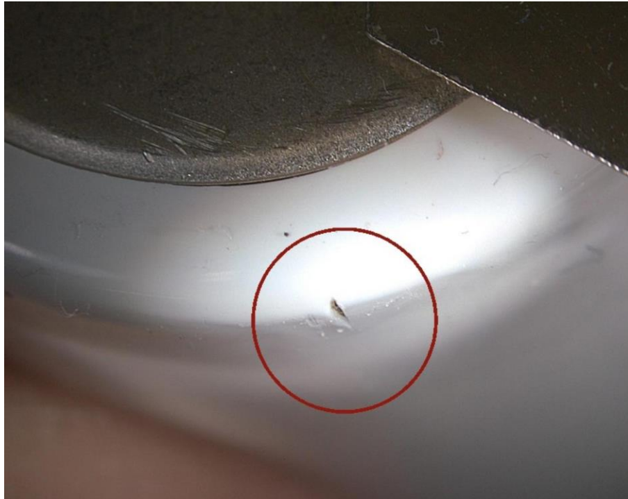
DEFECTIVE CELL INSULATION: EXAMPLE 3 FIGURE 5004
