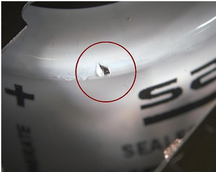
DEFECTIVE CELL INSULATION: EXAMPLE 2 FIGURE 5003
